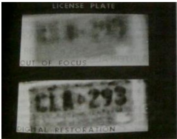
Fig: A blurred photograph of a license plate becomes legible after the application of image processing techniques.
